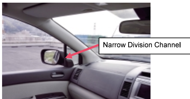
Fig.20 Triangle Window and Division Channel
