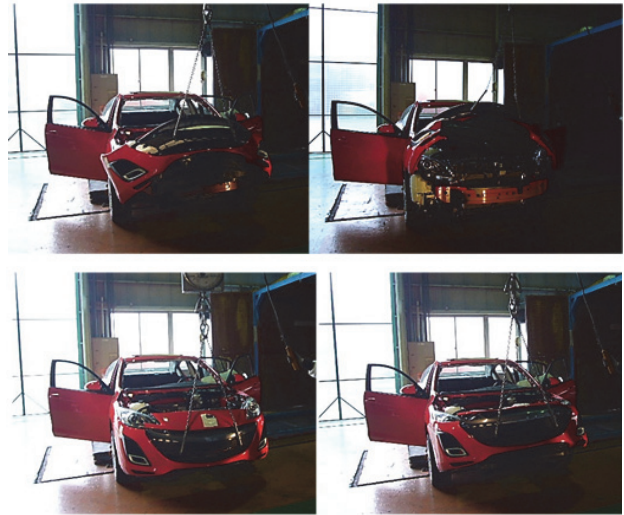
Fig. 9 Dismantlement Test of Bumper Designed for Recycling
