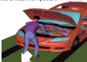
Fig.3 Double Slat Conveyor (Conventional)
