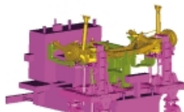
Fig.9 Rear Suspension Assembly to Accommodate Multi-Models
