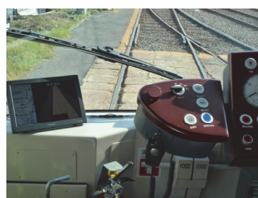
Fig. 11 Support Monitor for Tramcar
