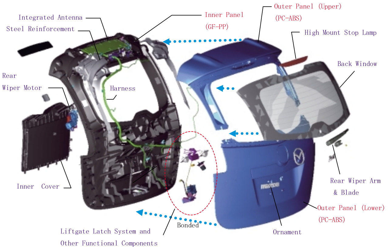
Fig.1 Basic Structure of Liftgate Module
