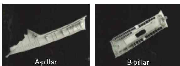
Fig.14 Energy Absorb Structure of Pillars
