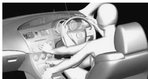
Fig.3 Zone Layout Concept (Operation)
