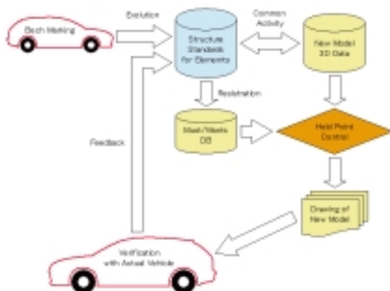
Fig.5 Process Flow for Standard Structure of Elements
