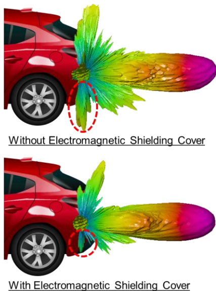
Fig. 11 Effect of Electromagnetic Shielding Cover
