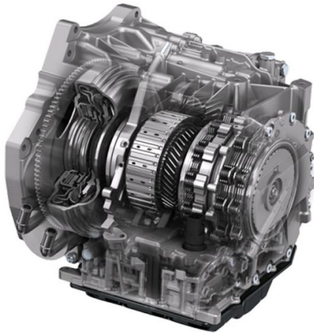
Fig.1 Phantom View of SKYACTIV-DRIVE
