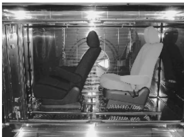
Fig.5 Test Equipments (2m 3 Chamber)
