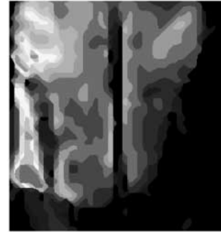
Fig.4 Front Seat Back Holding Performance at Cornering
