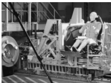
Fig.1 Side Impact Crash Simulator
