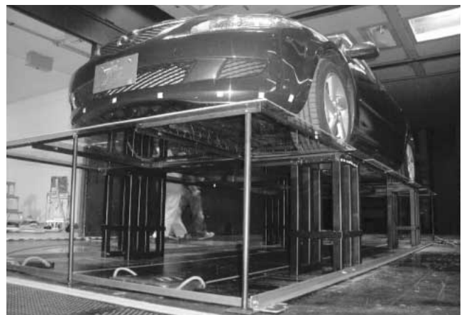
Fig.3 Equipment for Under Floor Flow Analysis
