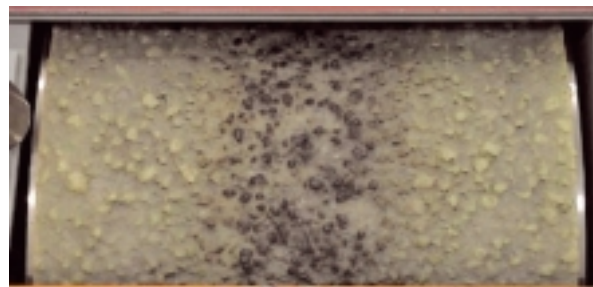
Fig.6 Course Road Noise Chassis Dynamometer
