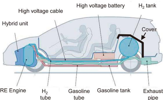
Fig.7 Layout of H<sub>2</sub> Tank
