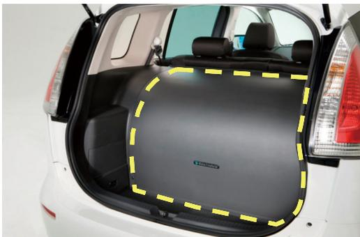
Fig.12 H<sub>2</sub> Tank Cover on Premacy Hydrogen RE Hybrid
