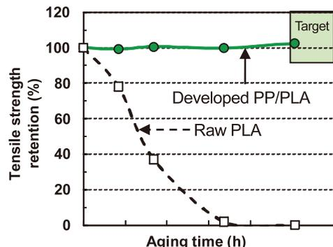
Fig.6 Tensile Strength Retention After Hydrolysis Test
