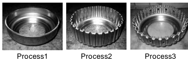
Fig.1 Clutch Drum Forming Process
