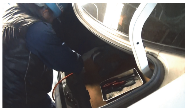
Fig. 6 Dismantlement Test 3 of Rear Bumper of Mazda Familia (Removed Fastening Bolts)
