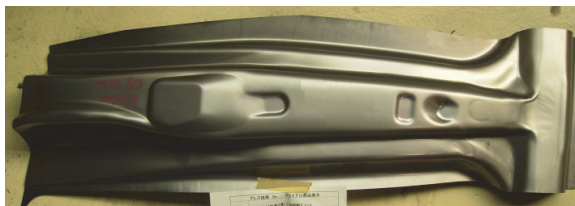
Fig. 2 Stamped Panel of Experiment
