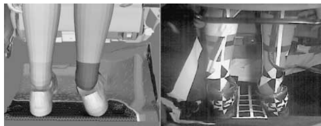
Fig.9 Comparison of the Dummy Lower Leg Kinematics at 90ms
