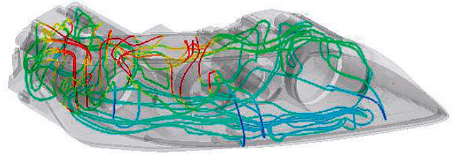
Fig.5 Streamlines Inside Headlamp Unit
